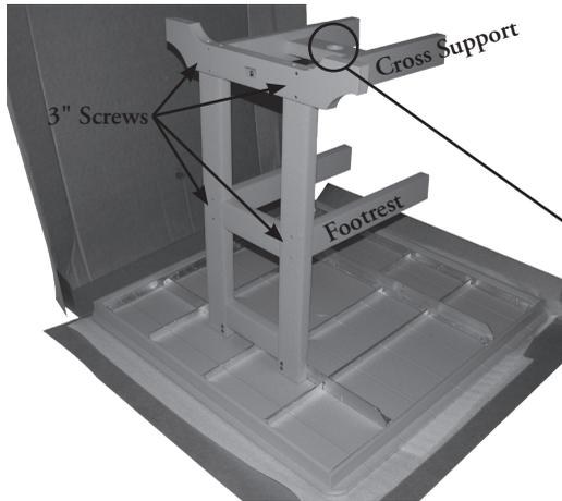
STEP #2 - First fasten the Cross Support to the Base using 3" Screws. Second fasten the two Footrests to the Upright using 3" Screws (Bar and Counter height only).
