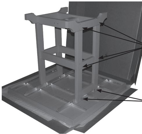
STEP #3 - First fasten the second Base to the aluminum frame of the Top using 1/4" x 2" Allen Head Bolts. Second fasten the Cross Support and Footrests to the Base using 3" Screws.
