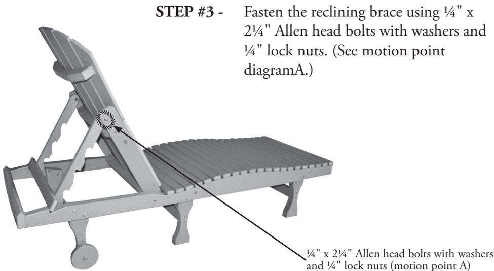
**STEP #3 -** Fasten the reclining brace using 1/4" x 2 1/4" Allen head bolts with washers and 1/4" lock nuts. (See motion point diagram A.)
