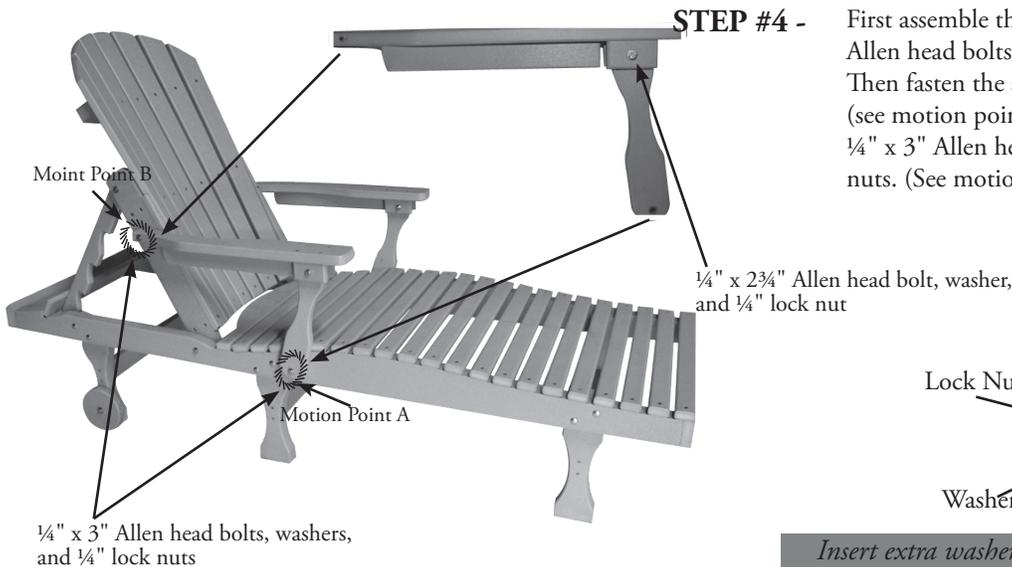
**STEP #4 -** First assemble the arm assembly using 1/4" x 2 3/4" Allen head bolts, one washer, and 1/4" lock nuts. Then fasten the arm assembly to the seat support (see motion point diagram A) and the back using 1/4" x 3" Allen head bolts, washers, and 1/4" lock nuts. (See motion point diagram B.)
