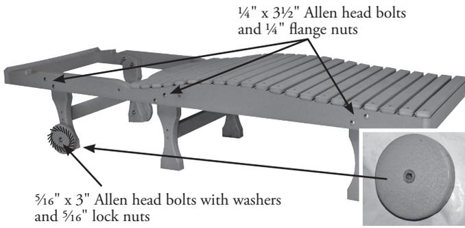
**STEP #1 -** Fasten the three leg assemblies to the seat using 1/4" x 3 1/2" Allen head bolts and 1/4" flange nuts. Then attach the wheel using 5/16" x 3" Allen head bolts, washers, and 5/16" lock nuts. (See motion point diagram A.)
