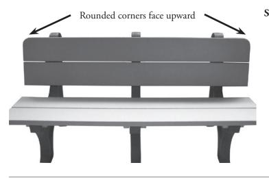
Step #3 Place back boards against leg uprights, fitting uprights between vertical supports on rear of back. Ensure that rounded corners face upward. Fasten using 12-2½" screws.
